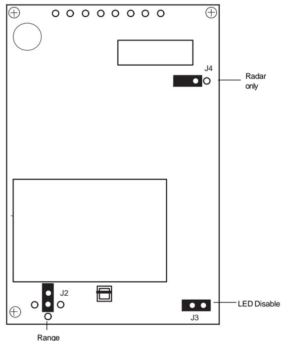
Figure 4. Main Circuit Board
