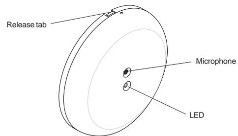
Figure 4. Housing Parts
