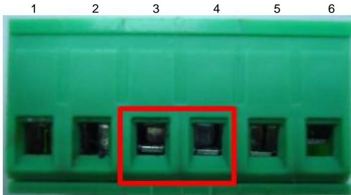
Insert the wires into the fault alarm contacts.
