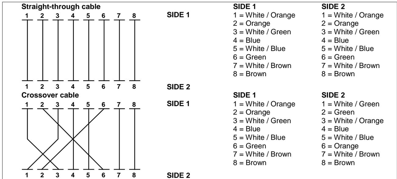
Ensure that the connected cables have the same pin assignment and color as described above.
