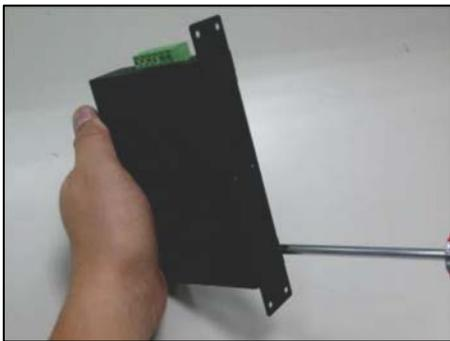
3. Use the screws to screw the wall-mount plate on the industrial fast Ethernet switch.
