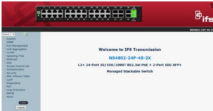
Figure 9: Web Main Screen of Web Smart PoE Switch
