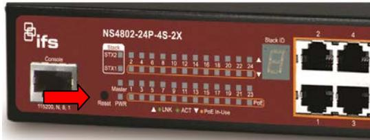
Figure 11: Stackable PoE Managed Switch Reset Button
