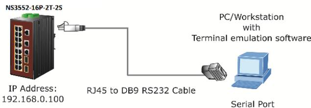
A terminal program is required to make the software connected to the industrial managed switch. Windows' Hyper Terminal program may be a good choice. The Hyper Terminal can be accessed from the **Start** menu.
