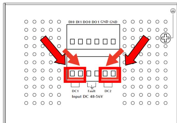
2. Tighten the wire-clamp screws to prevent the wires from loosening.
