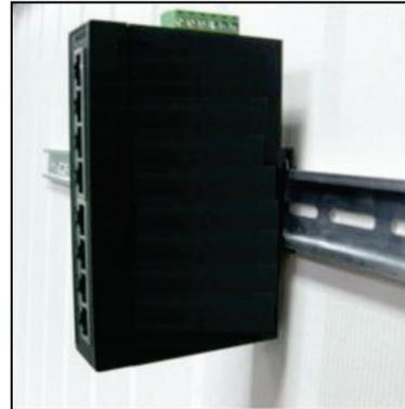
To remove the industrial gigabit Ethernet switch from the track, carefully pull out the bottom of the DIN-rail to remove it from the track.
