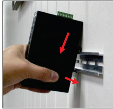
3. Ensure that the DIN-rail is secured to the track.
