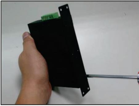
3. Use the screws to screw the wall-mount plate on the industrial gigabit Ethernet switch.
