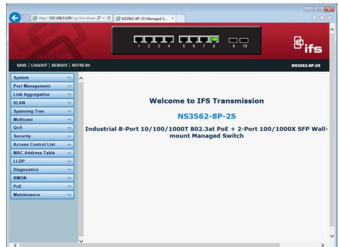
The switch menu on the left side of the Web page permits access to all of the commands and statistics provided by the wall-mount managed switch.
