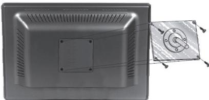
The monitor's installation surface is compatible with other types of VESA standard stands.
