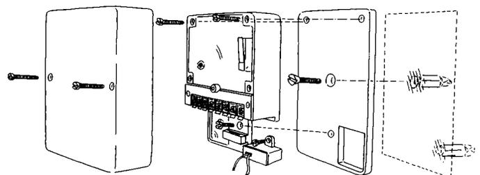
1. Define the exact location of the DV1201/DV1221 and hold the mounting plate to the wall.
