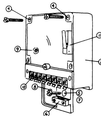
Removing the cover screws and cover from the base plate (2) provides access to the connection terminals (10) and the sensitivity adjustment control (9).
