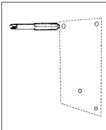
2. Using the felt pen and the mounting plate as a template, mark the location of the three threaded holes (see holes marked "V" in figure 9).
