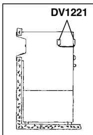
body, a DV1201 can be mounted on the outside surface or a DV1221 can be mounted on the inside metal surface.
