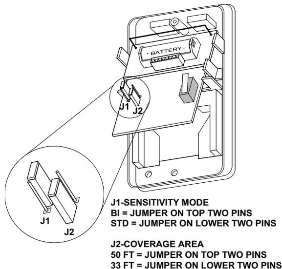
Figure 7. Sensitivity Mode and Coverage Area Jumper Settings
