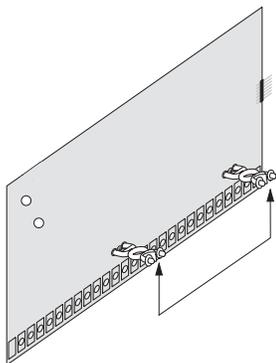
4. Slide the top of the backplates onto the left and center module mounting clips on the panel cabinet ([Figure 4](#)),
