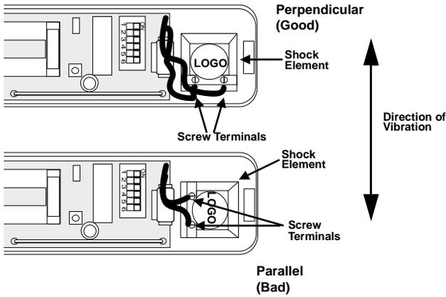
**Figure 4. Positioning shock elements for horizontal surface mounting**
